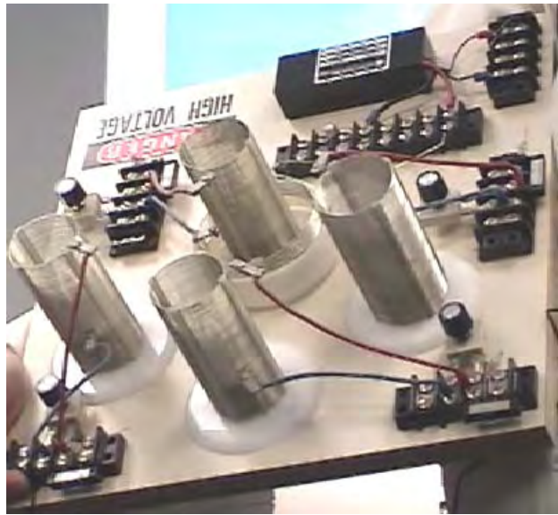
The "L1" short outer coil is held in a raised position by the section of white plastic pipe in order to position it correctly relative to the smaller diameter "L2" secondary coil. Again, it appears to have five turns:
